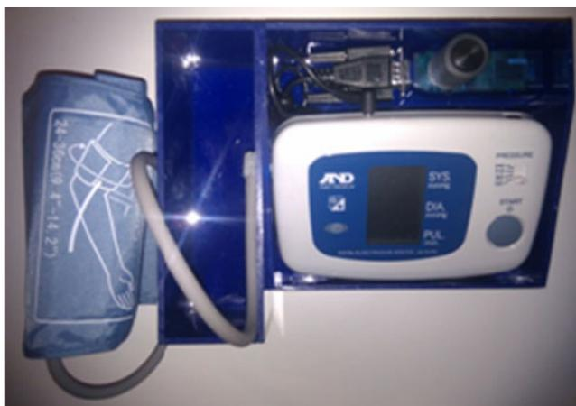
**Fig. 5** Designed Bluetooth-enabled blood pressure monitor
